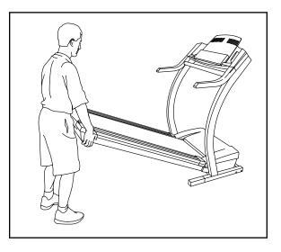
2. Move your right hand to the position shown and hold the treadmill firmly. Using your left hand, pull the latch knob to the left and hold it. Raise the treadmill until the frame is past the latch pin. Slowly release the latch knob. **Make sure that the frame is securely held by the latch pin.**
